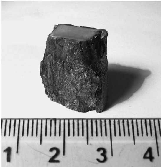
Fig. 4. A TE-processed billet with dimensions of about 14 mm × 23 mm × 40 mm compacted at 523 K from amorphous \text{Al}_{86}\text{Gd}_6\text{Ni}_6\text{Co}_2 melt-spun ribbons.
